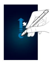
On the Quick Command screen, draw a gesture command to launch the assigned application or feature. To view assigned gesture commands, press the S Pen button while hovering over the Quick Command screen.
